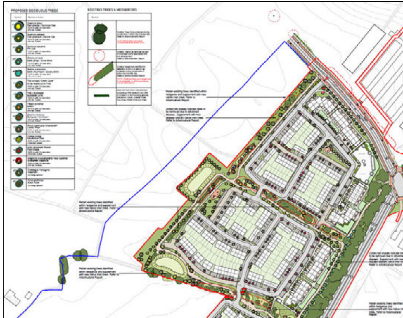
FIGURE 16. EXTRACT FROM THE PLANTING PLAN SHOWING SUPPLEMENTARY PLANTING OF AFFECTED HEDGEROWS (SOURCE: IRLA DRWG No: 5000)
